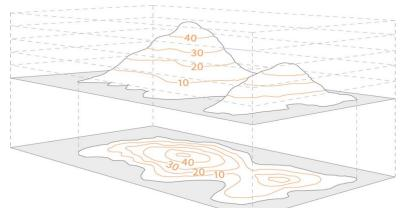
You can see from the picture above the link between the shape of a hill and the contours representing it on a map. Another way of thinking about contour lines is as a tide mark left by the sea as the tide goes out, leaving a line every 5 metres.
